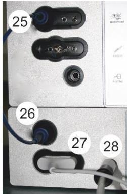
Connect the monopolar output (25) of the HF-device to the input of the Argon module (26).
