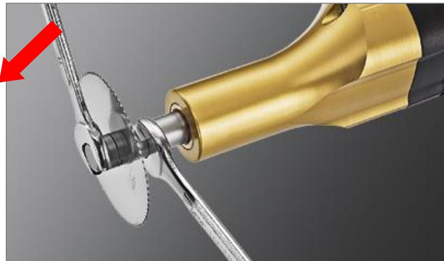
**fig. 3 Releasing the retaining screw**
